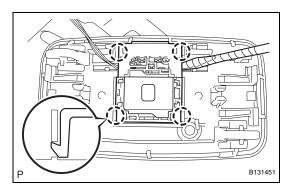
(d) Using a screwdriver, detach the 4 claws and remove the room light switch base. HINT:
