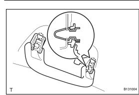
12. INSTALL REAR ASSIST GRIP ASSEMBLY (a) Attach the 4 claws to install the assist grip.
