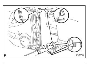
53. INSTALL LOWER CENTER PILLAR GARNISH LH(a) Attach the 2 claws and 2 clips to install the garnish.
