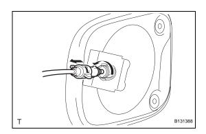
(c) Turn the lock retainer counterclockwise and remove the cable from the retainer.
