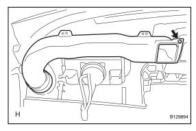
8. INSTALL NO. 1 HEATER TO REGISTER DUCT
