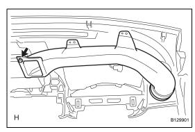
3. REMOVE NO. 1 HEATER TO REGISTER DUCT
