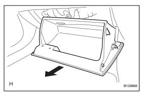
(e) Pull the glove compartment door toward the rear of the vehicle to detach the 2 hinges and remove the glove compartment door.
