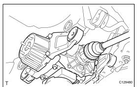
(c) Slowly lower the jack and then tilt the rear differential carrier as shown in the illustration.
