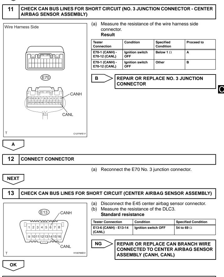
REPLACE CENTER AIRBAG SENSOR ASSEMBLY
