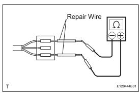
(b) Use a repair wire to check the connector if it is impossible to check resistance from the rear of the connector.
