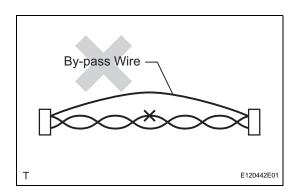
(b) Do not use bypass wiring between the connectors. **NOTICE:**
