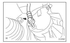
(e) Remove the union bolt and gasket(s), and then remove the flexible hose from the disc brake cylinder.
