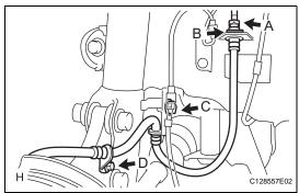
(d) Tighten the bolt (labeled C) to fix the flexible hose clamp and sensor clamp.
