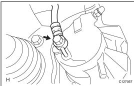
(a) Connect the flexible hose with new gasket(s) and the union bolt to the disc brake cylinder.
