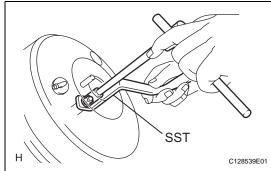
(c) If the clearance is not within the standard, adjust the length by holding the rod using SST and turning the tip of the rod using a 7 mm socket driver.
