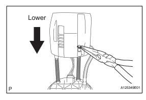
(b) Using needle nose pliers, remove the E-ring.HINT:Slightly lower the sub-tank to remove the E-ring.
