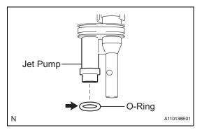
(g) Remove the O-ring from the jet pump.
