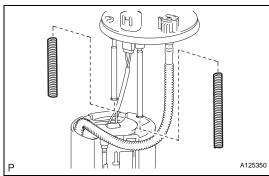
(c) Remove the 2 springs from the 2 shafts.
