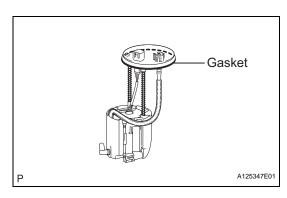
(b) Remove the gasket from the fuel pump.
