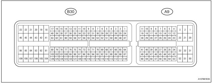
(a) Measure the voltage of the ECM connector. HINT:
