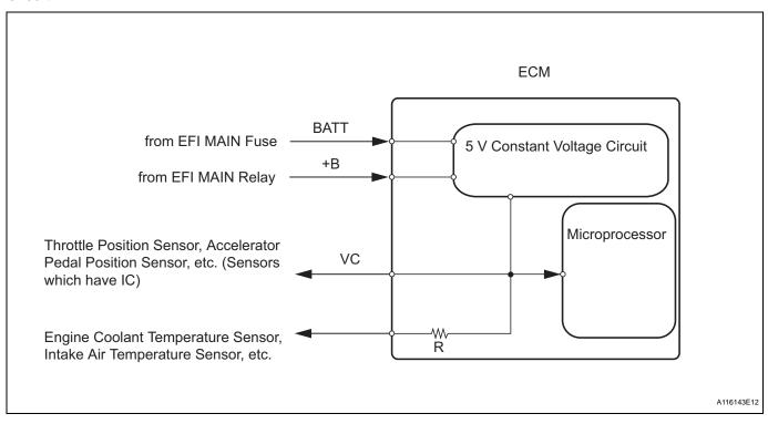
When the VC circuit is short-circuited, the microprocessor in the ECM and sensors that are supplied with power through the VC circuit are inactivated because the power is not supplied from the VC circuit. Under this condition, the system does not start up and the MIL does not illuminate even if the system malfunctions.
