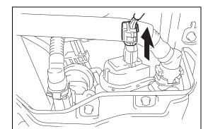
(a) Disconnect the S3 canister pump module connector.(b) Turn the ignition switch ON.
