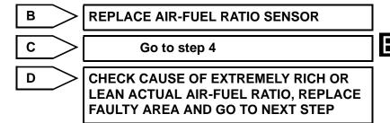
Α 3 CHECK FOR EXHAUST GAS LEAKAGE OK: No gas leakage. NG **REPAIR OR REPLACE EXHAUST GAS** LEAKAGE POINT OK **REPLACE THREE-WAY CATALYTIC CONVERTER (BOTH FRONT AND REAR CATALYSTS** (FRONT EXHAUST PIPE)) 4 CHECK FOR EXHAUST GAS LEAKAGE OK: No gas leakage. NG **REPAIR OR REPLACE EXHAUST GAS** LEAKAGE POINT OK
