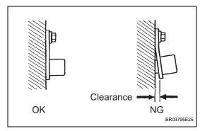
(a) Check the CKP sensor installation.
