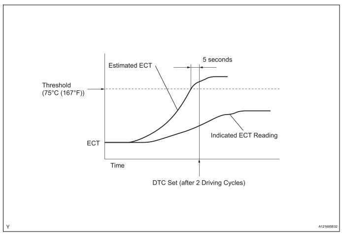
The ECM estimates the ECT based on the starting temperature, engine loads, and engine speeds. The ECM then compares the estimated temperature with the actual ECT. When the estimated ECT reaches 75°C (167°F), the ECM checks the actual ECT. If the actual ECT is less than 75°C (167°F), the ECM interprets this as a malfunction in the thermostat or the engine cooling system and sets the DTC.
