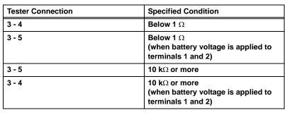
If the result is not as specified, replace the relay.
