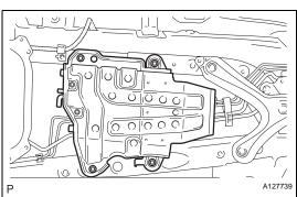
(b) Remove the 4 bolts, clip and canister.
