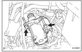
(c) Remove the 2 bolts and starter.
