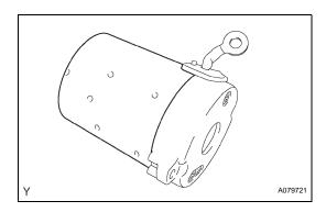
(b) Remove the starter yoke from the commutator end frame.
