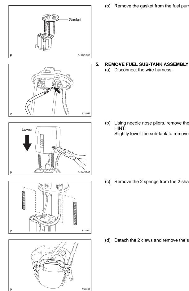
(b) Remove the gasket from the fuel pump.
