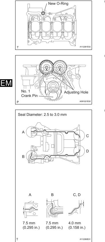
(b) Place a new O-ring on the cylinder block as shown in the illustration.
