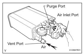
(2) While holding the air inlet port closed, blow air 0.39 kPa (4.0 kgf/cm², 3 mmHg) into the vent port, and check that air flows from the purge port.
