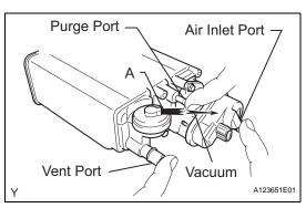
(3) While holding the vent, purge and air inlet ports closed, apply vacuum 1.42 kPa (14.5 kgf/cm², 10.6 mmHg) to port A, and measure how long it takes for the vacuum to drop.
