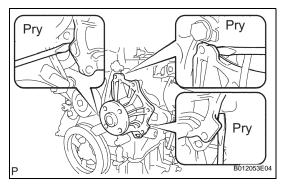
(d) Using a screwdriver, pry between the water pump and cylinder block, and then remove the water pump.
