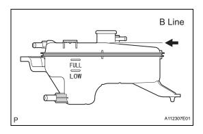
(d) Continue adding TOYOTA SLLC until it is filled to the B line at the base of the reservoir's filler neck. HINT:
