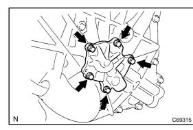
(b) Apply liquid sealant 1344 to the first 2 or 3 threads of the bolt end.
