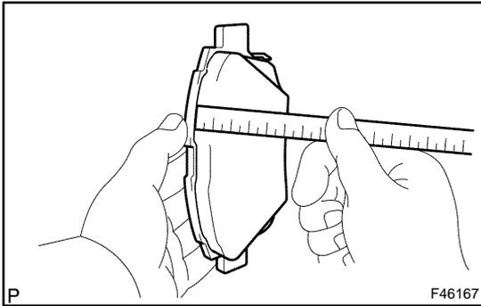
**18. INSPECT PAD LINING THICKNESS**
