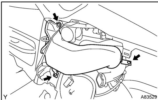
12. REMOVE VENTILATOR DUCT INNER
