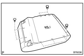
(e) Using a clip remover, remove the 7 clips.
