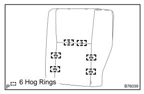
(i) Remove the 6 hog rings and cover from the rear seatback pad.
