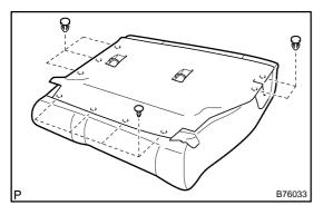
(f) Using a clip remover, remove the 9 clips.
