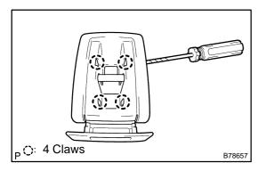
(e) Using a screwdriver, disengage the 4 claws and remove the 2 rear seat back covers.
