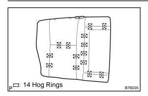
(j) Remove the 14 hog rings and cover from the rear seatback pad.
