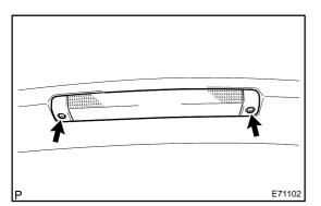
(c) Remove the 2 screws and the center stop lamp assy. **NOTICE:**
