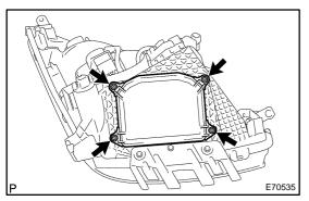
9. REMOVE HEADLAMP LIGHT CONTROL COMPUTER SUB-ASSY (DISCHARGE HEAD LAMP)
