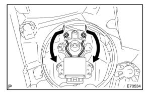
(c) Push the set spring in the direction indicated by the arrow in the illustration and remove the discharge headlamp bulb.
