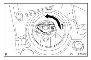
(b) Push the set spring in the direction indicated by the arrow in the illustration to remove the headlamp No.1 bulb.
