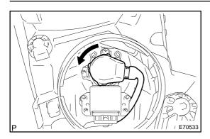
(b) Turn the headlamp light control computer socket in the direction indicated by the arrow in the illustration to remove it.
