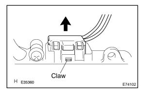
(c) Disengage the claw and disconnect the connector, and then remove the headlamp light control computer subassy.
