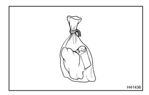
(h) Dispose of the front passenger airbag assy.
