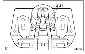
(d) Using a service–purpose wire harness for the vehicle, tie down the front passenger airbag assy to the tire.
