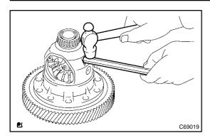
(g) Using a chisel, calk the external circumference of the differential case straight pin hole.
