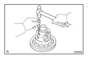
(f) Drive the straight pin into the differential case with a pin punch (5 mm).
