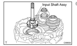
(g) Install the input shaft assy.
