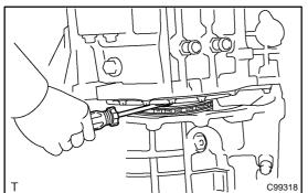
(g) Apply protective tape to the head of a flat-head screwdriver and use it to hold down the chain with input shaft assy while removing the generator assy.
