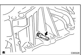
(b) Apply liquid sealant 1344 to the first 2 to 3 threads of each of the 6 bolts. Install the motor water jacket cover with the 6 bolts.
