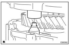
(b) Install the parking lock rod to the generator assy so that it is inserted into the cam guide sleeve. Use an engine sling device and chain block.
