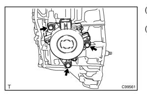
(b) Install the shift control actuator with the 3 bolts.
