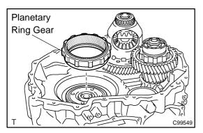
Install the planetary ring gear.
