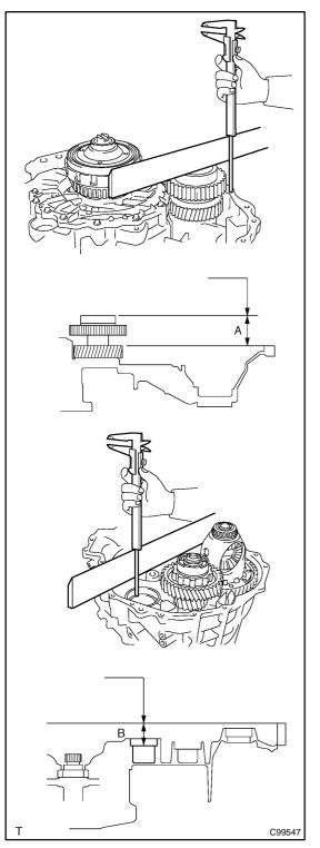
(2) Using a straight edge and vernier calipers, measure dimension A as shown in the illustration.
