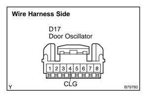
(a) Measure the frequency between the terminals of the connector when the power switch is operated.
