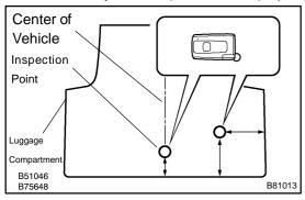
(2) Inspect the smart key lock—in prevention's detection area. Pay attention to the direction of the smart key in the illustration on the left. When the smart key is in either of the two locations in the illustration, check that: 1) closing the back door sounds the smart key's wireless buzzer, and 2) pressing the luggage electrical key switch (trunk switch) opens the back door.
