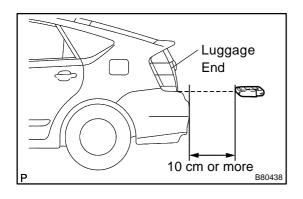
(3) Inspect the smart key lock—in prevention's detection area and the trunk interior's wireless door lock receiver for wave leaks. Hold the smart key at the same height as the lower edge of the back door and aligned with the center of the rear of the vehicle. Pay attention to the direction and position of the smart key in the illustration on the left. Check that when the smart key is over 10 cm (0.6 ft) from the vehicle's rear bumper, the smart key's wireless buzzer does not sound.
