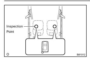
(3) Inspect the smart ignition operation's detection area. Pay attention to the direction of the smart key in the illustration on the left. When the smart key is in either of the two locations in the illustration, check that the engine can start.
