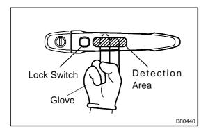
(5) Inspect the door oscillator's response sensitivity. Wear protective gloves, set the system to unlock standby mode, and check that touching the inner side of the outside handle (the highlighted area in the illustration) with your index finger causes the door to unlock.
