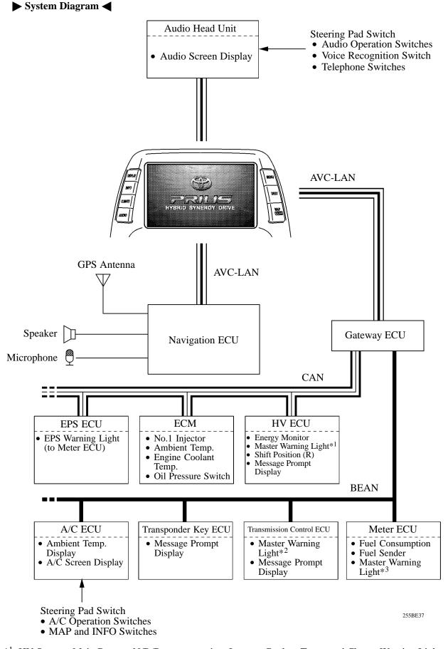
\*1: HV System, Main Battery, N/D/B range warning, Inverter Coolant Temp. and Charge Warning Light
