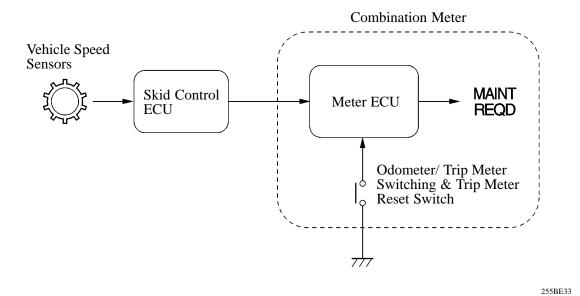
• After the engine oil has been changed, accumulated vehicle driving distance memorized in the meter ECU should be reset by the odometer/ trip meter switching & trip meter reset switch. At this point, the accumulated vehicle driving distance is reset to zero and the cycle begins again.
